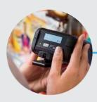
Easy to use Mono LCD and three flat membrane keys.
